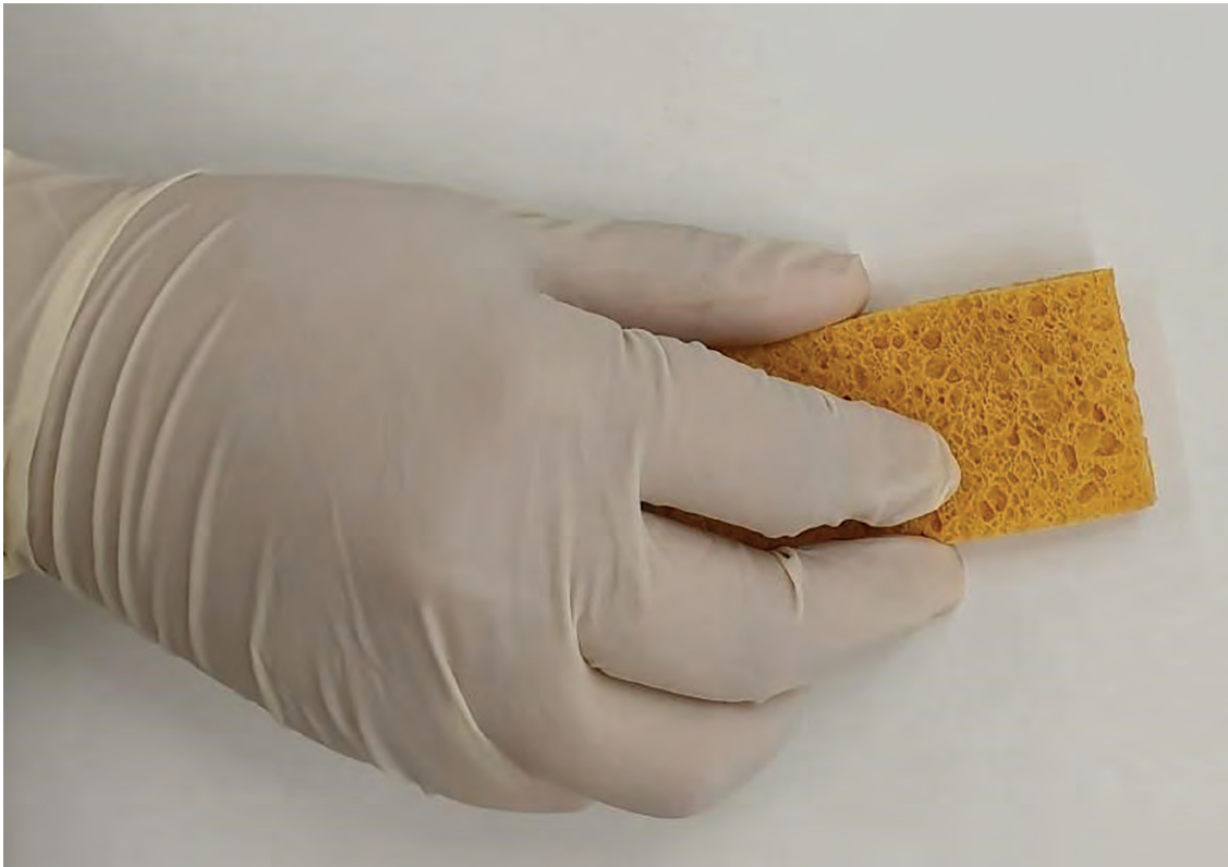
Figure 49. Sponges are recommended for general sampling using sterile gloves.
