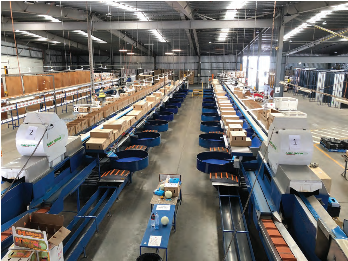
Figure 46. A typical packhouse environment showing packing tables and conveyor belts where microbial pathogens can survive and form biofilms.
