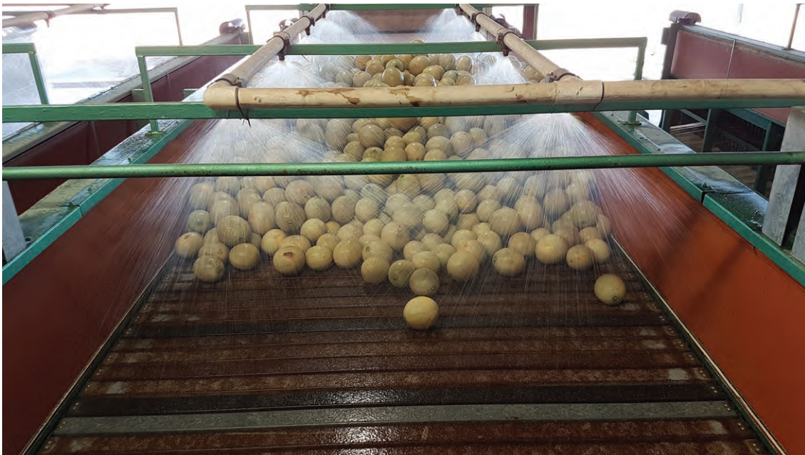
Figure 26. Rinsing melons before they are washed and sanitised.
