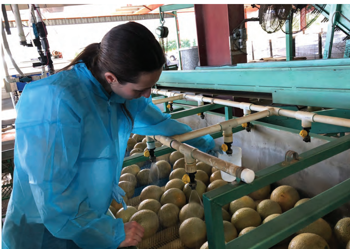
Figure 29. Wash water sampling and monitoring.
