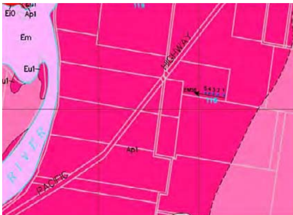
Figure 18. Five K_{sat} pits and an EM38 transect. (source: Naylor et al., 1998)
