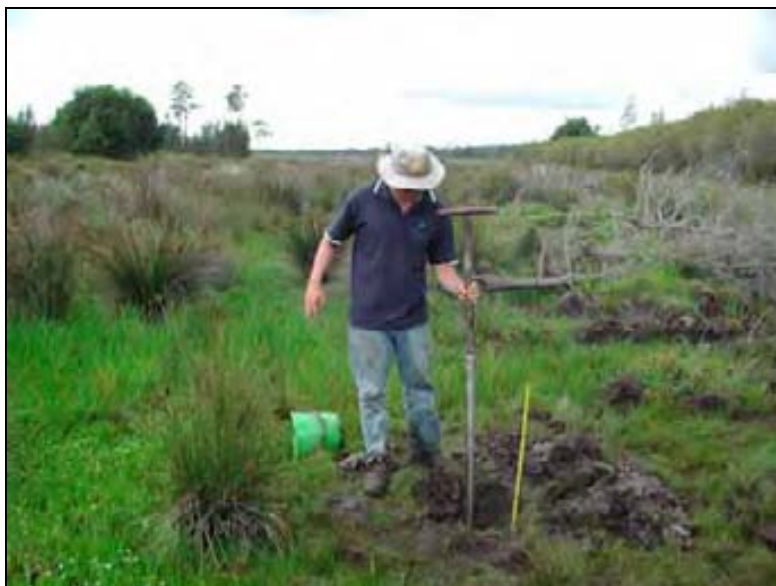
Figure 5. Thor Aaso using a gouge auger in a K_{sat} pit, in the Hastings.
