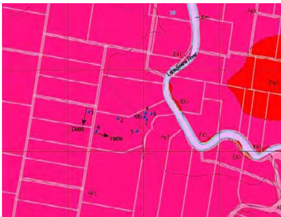
Figure 85. Eight K_{sat} pits and two EM38 transects, at Roches. (source: Naylor et al., 1998)
