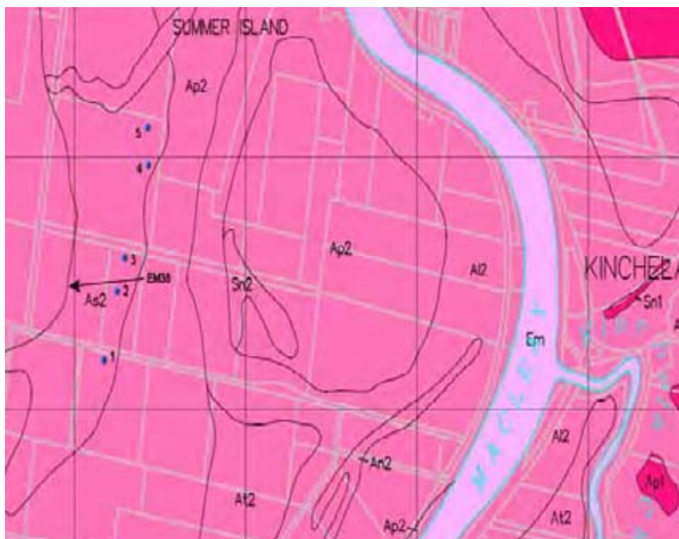
Figure 64. Five K sat pits and an EM38 transect. (source: Naylor et al., 1998)
