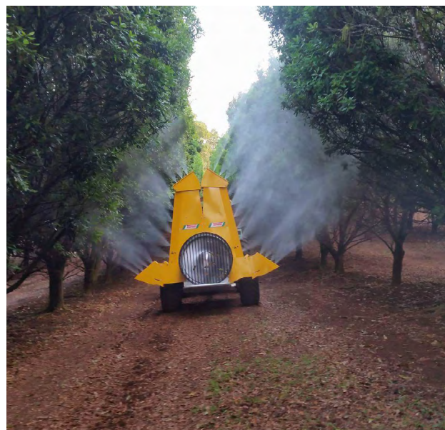
Figure 5. An Air SERGII Tower sprayer. Photo: Paul Blasutto, Tornado Sprayers.
