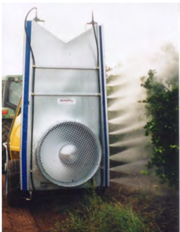
Figure 4. TPD assist tower sprayer. Photo: Paul Blasutto, Tornado Sprayers.
