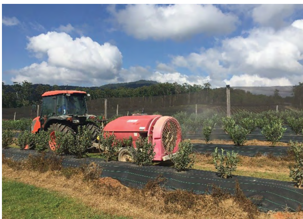
Figure 1. An axial air-blast sprayer. Photo: Melinda Simpson.
