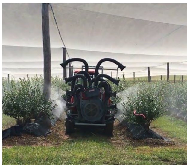
Figure 7. Assessing the sprayer output is towards the canopy. Photo: Melinda Simpson.
