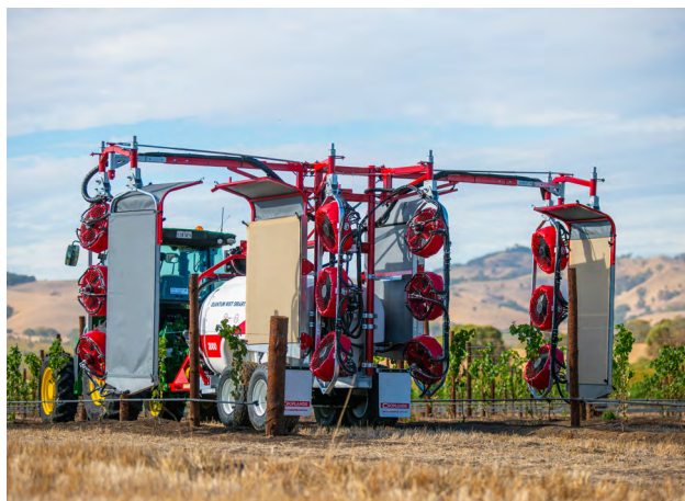
Figure 3. A recycling sprayer. Photo: Dave Farmer, Croplands.
