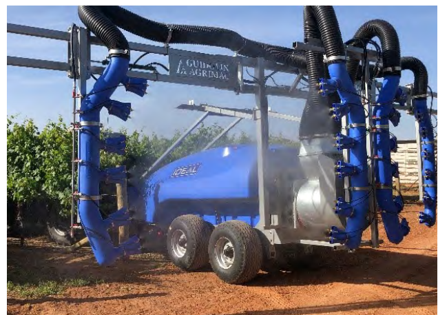
Figure 2. A multi-head sprayer. Photo: Marcel Guidolin, Guidolin Agrimac.
