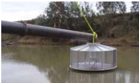
Research is continuing into the effective use of screens to minimise the impact of pumping on fish. Photo: NSW DPI.
