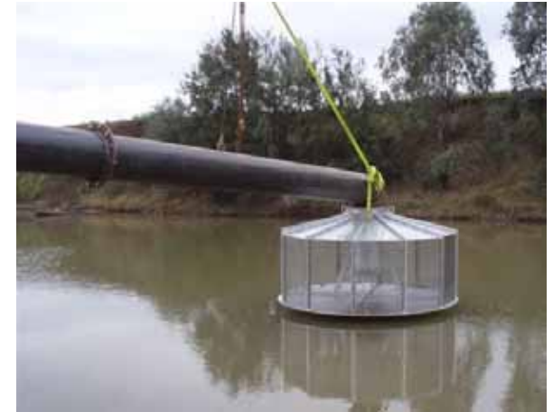
Research is ongoing to find out what sort of screens can be fitted to irrigation systems to minimise the damage to native fish populations. Photo: NSW DPI.
