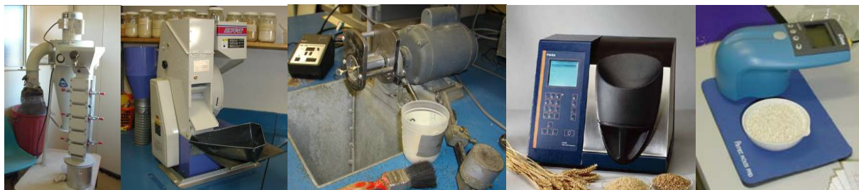
Figure 1. Physical quality assessment. From left to right: aspirator, dehuller, mill, image analysis and the spectrophotometer.
