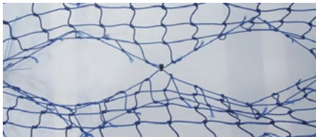
An entrance of a crab trap that has been reduced in size. The entrance is still big enough for all size crabs to enter.
