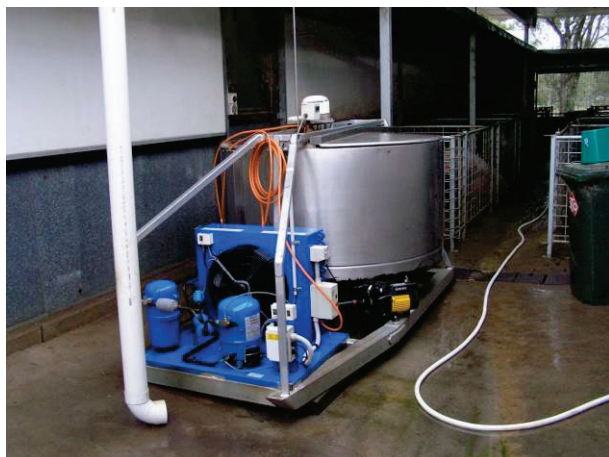
Figure 3: The mobile water chiller unit developed from a second hand milk vat.
