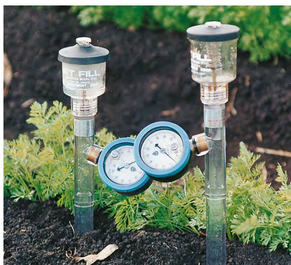
Figure 51. Tensiometers with ceramic tips and vacuum gauges.
