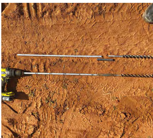
Figure 50. A soil auger can be built by welding a 200–300 mm wood auger drill bit onto a 12 mm rod.
