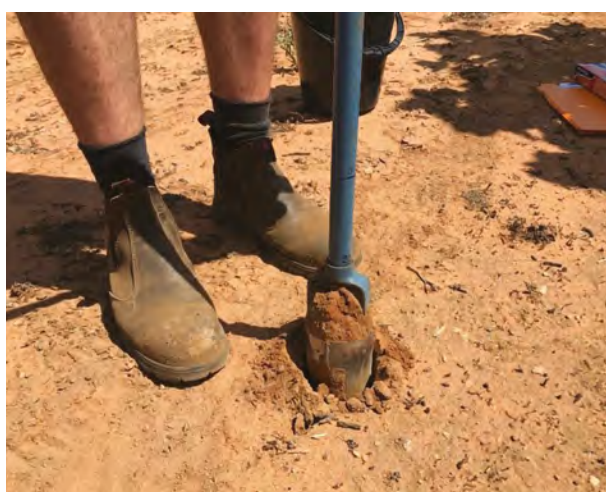
Figure 5. Soil sampling in Orange (NSW) with a hand auger.
