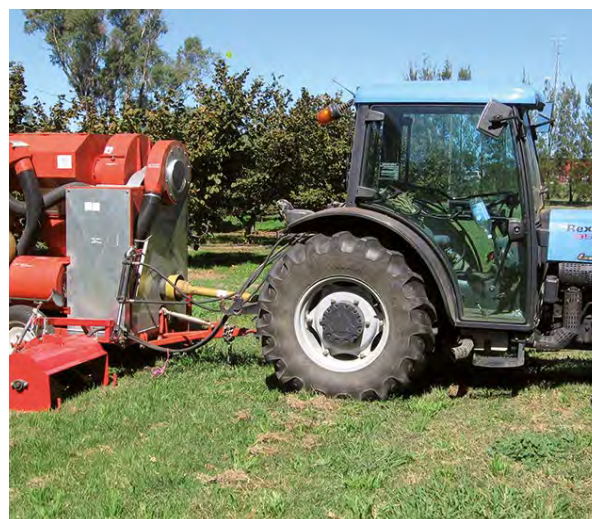
Figure 147. A vacuum harvester fitted with a side-mounted head.
