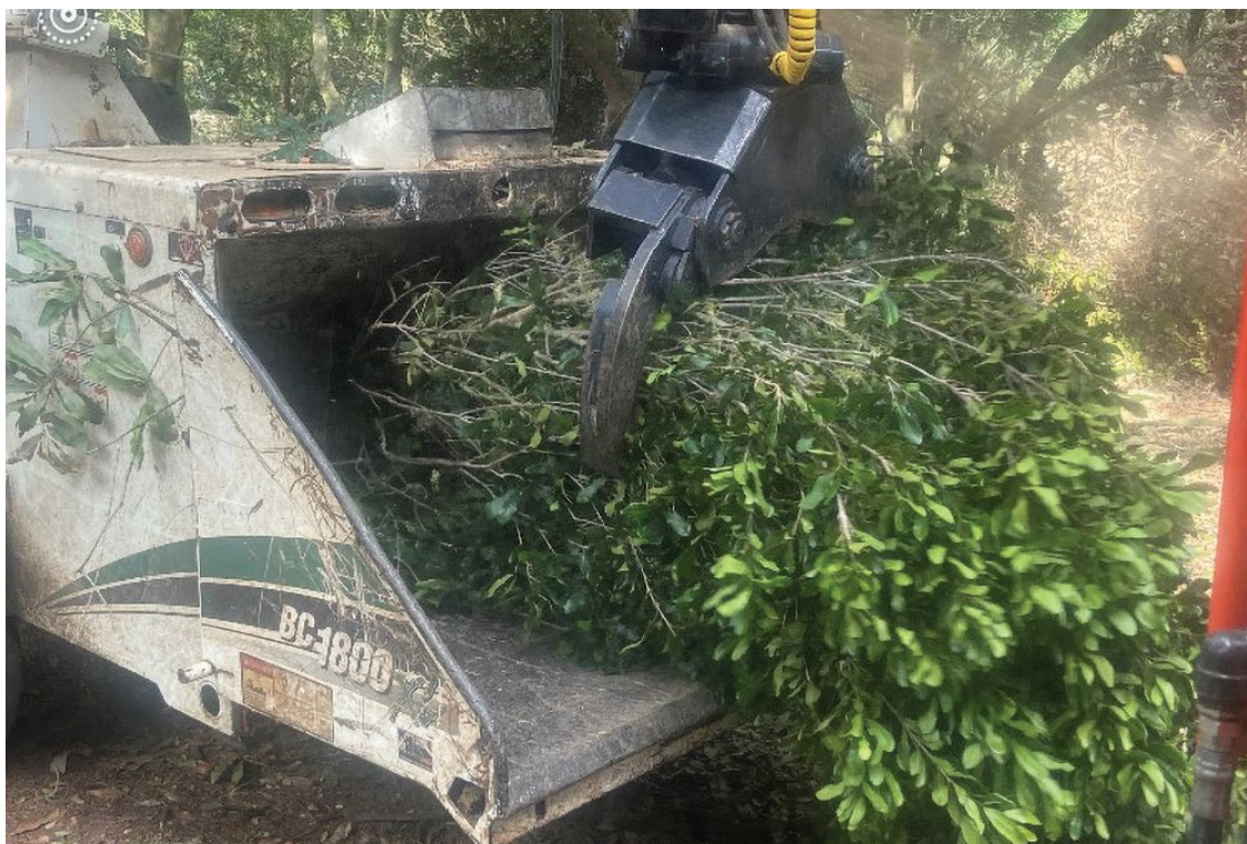
Figure 12. An excavator with a cut-and-grab attachment for pruning.
