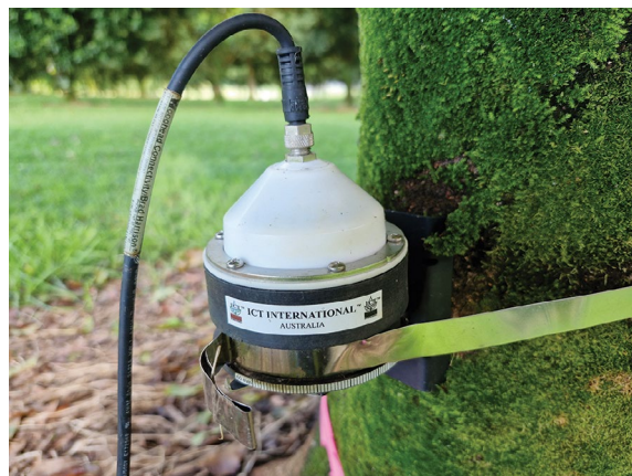
Figure 30. A dendrometer measuring trunk diameter.
