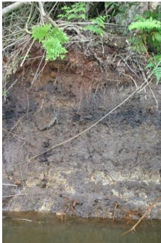
Figure 5 Yellow mottling of pyrite seen in the bank of the Main Drain, Anna Bay, above the drain water level. The dark band indicates evidence of previous peat fires (photo: S. Walsh)
