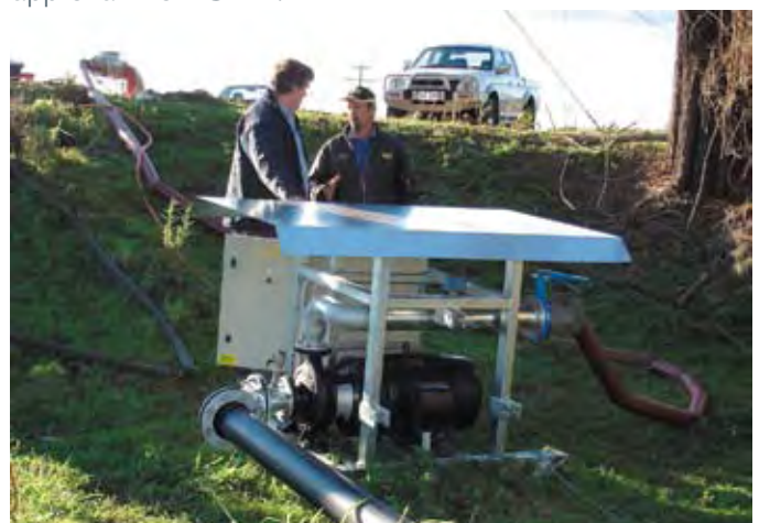
A skid mounted electric pump for irrigation from a river which floods.
