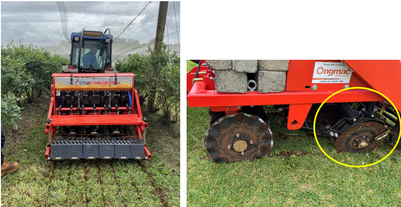
Figure 1. The Cosmo Bully® seven-disc direct drill seeder used to sow pollination/green manure mixes in blueberry inter-rows (left). Some features include a front cutting disc to slice through surface material and a seeding placement disc for accurate seed delivery (right).
