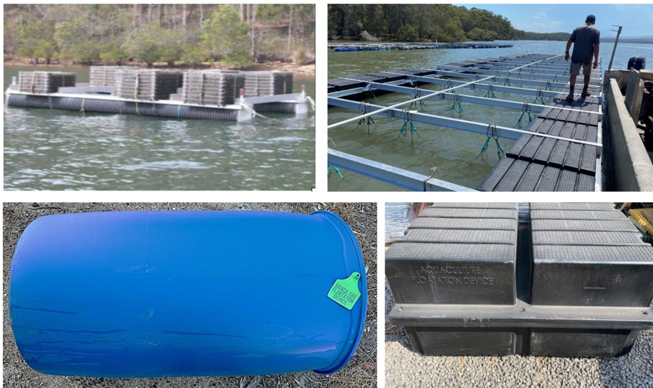
Figure 9. Examples of aquaculture floatation devices. An end-capped ribbed polyethylene pipe (top left). An aluminium raft with rota-moulded float providing a walking surface (top right). A food grade pickle drum used for timber rafts marked as an aquaculture floatation device using a cattle tag (bottom left). A rota mould aquaculture floatation device used on aluminium rafts and labelled during the manufacturing process (bottom right). Image source NSW DPIRD Aquaculture Management and Armstrong Oysters.
