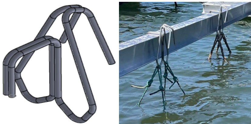
Figure 6. 3D isometric diagram of SS316 hooks (left). SS316 hooks being used to suspend oyster modules on an aluminium raft (right). Image source NSW DPIRD Aquaculture Management and Armstrong Oysters.
