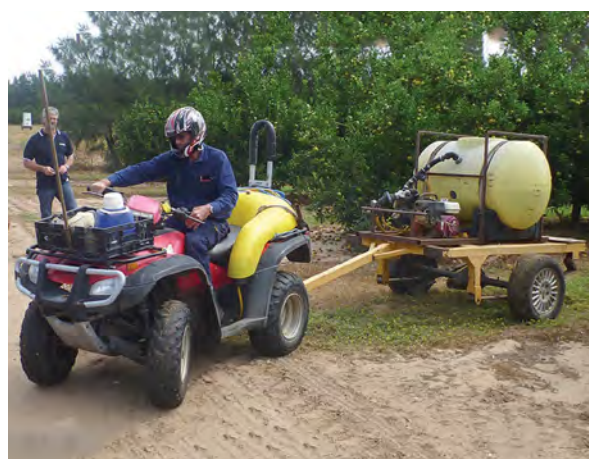
Figure 75. A quad bike towing a Queensland fruit fly spraying rig used by 2PH farms (Emerald). This rig enables higher water volumes to be carried than if using the bike without the tank.
