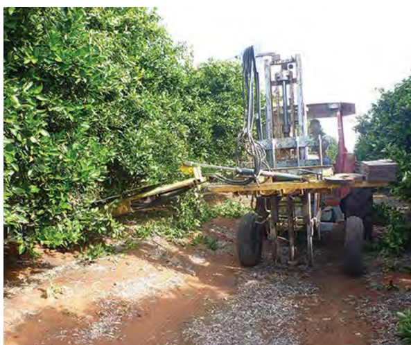
Figure 157. Skirting trees using a circular saw cutter bar mounted on the forks of a tractor.
