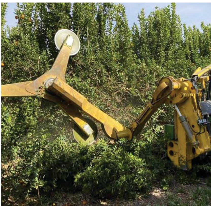
Figure 2. Using a mechanical hedging machine is a quick and inexpensive way to remove large portions of the tree's canopy, but will remove it indiscriminately.
