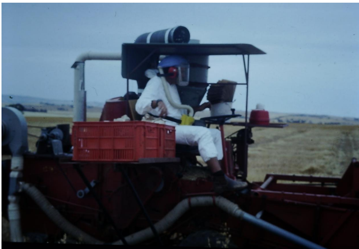
Figure 10; Around 1980, Portmann et al. modified the Hege harvester so that seed is delivered to the driver's side, allowing one man operation. Not surprising allergies became a problem, given the exposure to grain dusts
