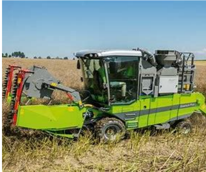
Figure 12 Contemporary Wintersteiger plot combine circa 2020 plot harvester featuring air-conditioned cabin, on board weighing of plots and sample collection.
