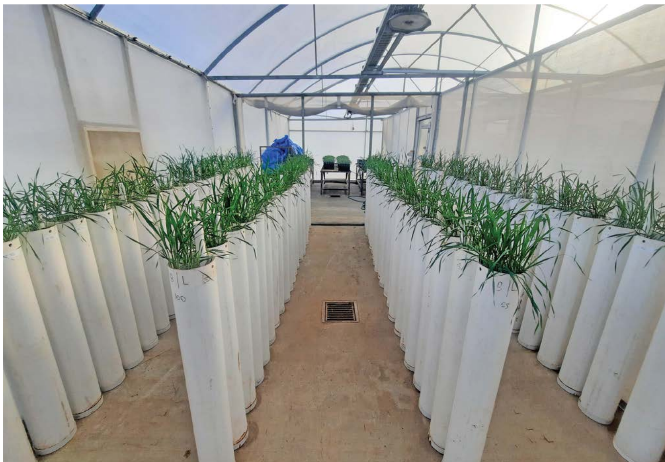
Figure 1 PVC tube design for controlled environment study exploring interactions between spatially (vertical) available soil N, FCR and available soil moisture during flowering.
