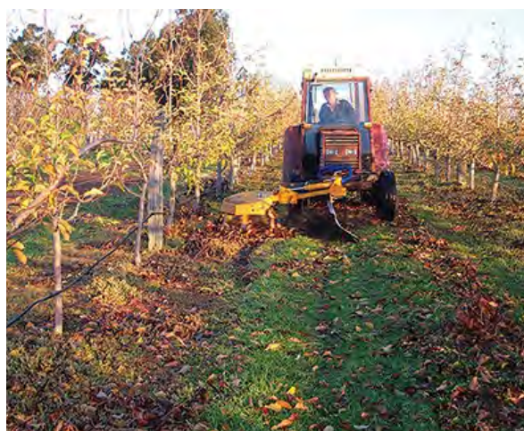
Figure 145. The Sadie sweeper moves leaf and pruning residue to the centre of the row for mulching. Photo: Crendon Machinery.
