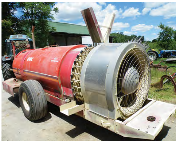
Figure 177. Deflectors on an air-blast sprayer. Photo: Deveau (2015).
