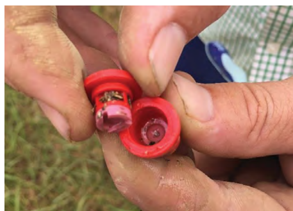
Figure 175. Regularly cleaning nozzles will improve delivery rates by removing debris build-up.
