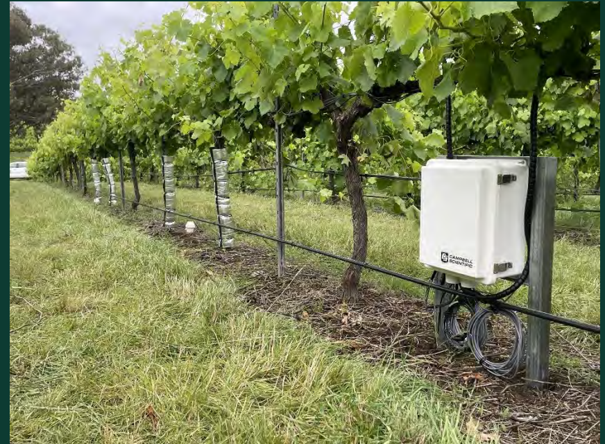
Sap flow gauges and automated soil moisture probe - 2021
