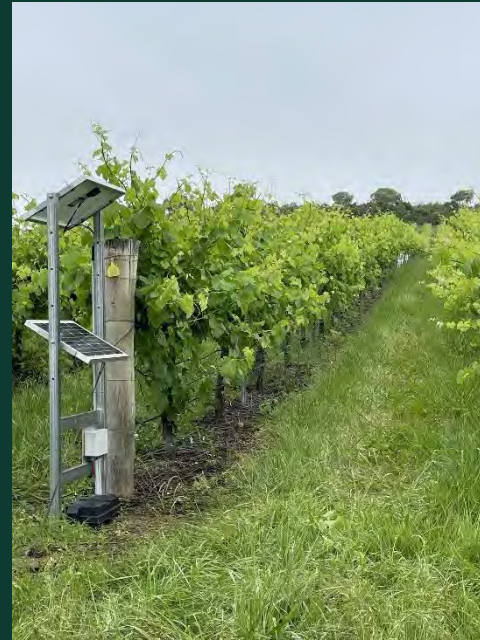
Sap flow gauges and automated soil moisture probe - 2021
