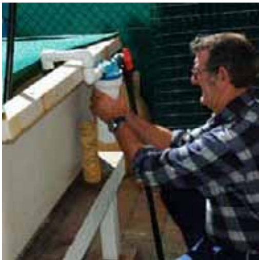
Figure 35 Nursery tank filter element being changed.
