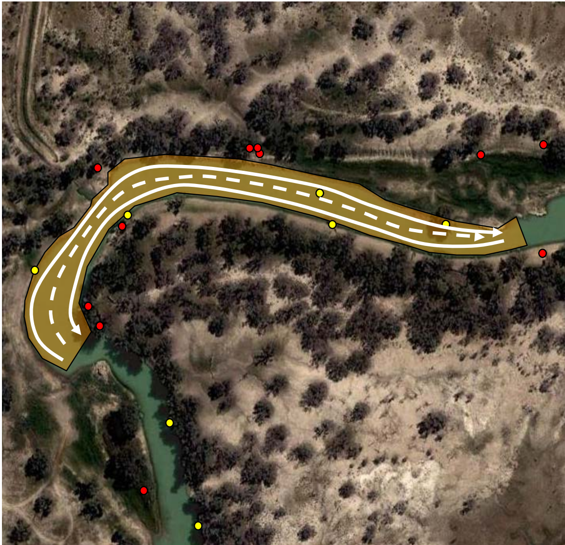
Figure 18. Electrofishing was conducted in 1080 continuous seconds of fishing effort at each site. The boat was moved along the left bank for 400 seconds, then down the right bank for 400 seconds, and finally up the middle of the channel for 280 seconds. Dots indicate low-flow available (red) and high-flow recruitable (yellow) large wood, as mapped in Chapter 3.
