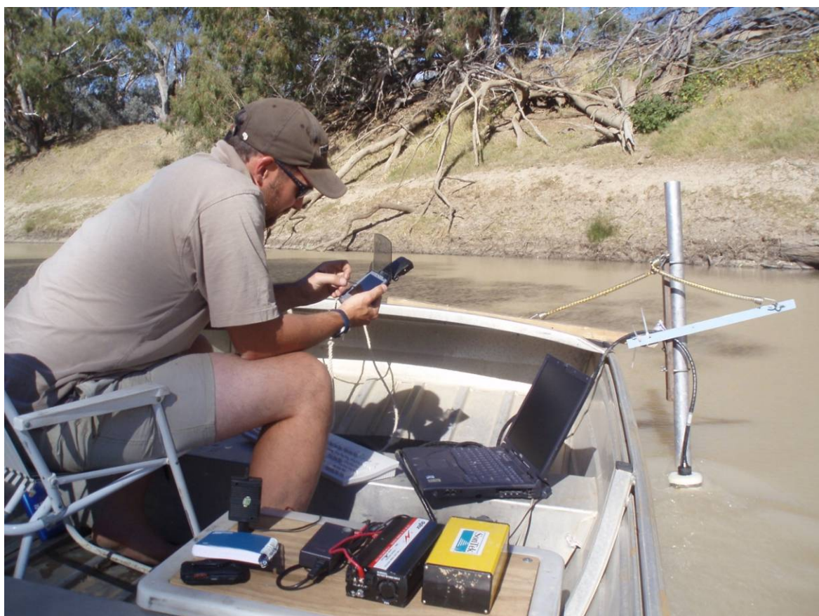
Figure 20. Surveys being undertaken with a boat-mounted ADP.
