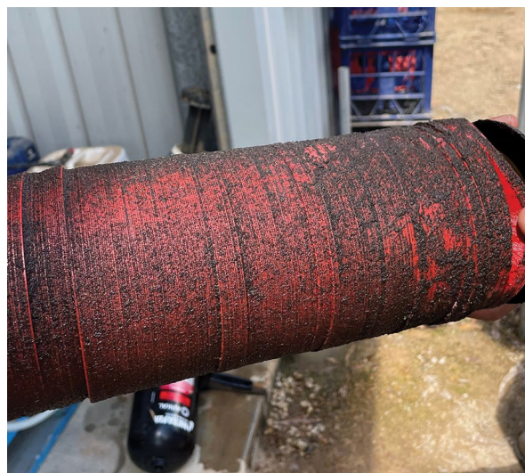
Figure 13. A dirty filter due to poor dam water quality.
