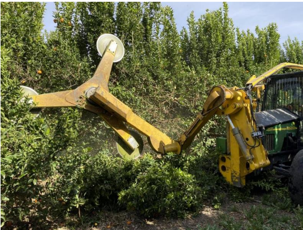
Figure 7. A mechanical hedging machine indiscriminately removes the canopy but is a quick and inexpensive method to cut large portions of the tree's canopy.
