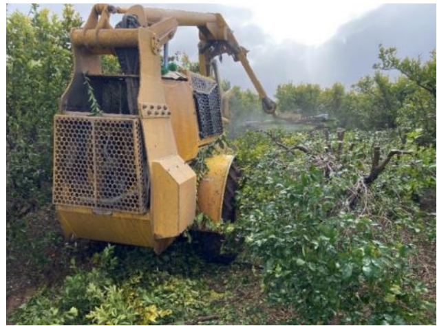
Figure 15. Left: the staggered double-row planting. Right: a mechanical hedging machine resetting the western side of staggered double-row planted trees by topping them at 1.6 m.
