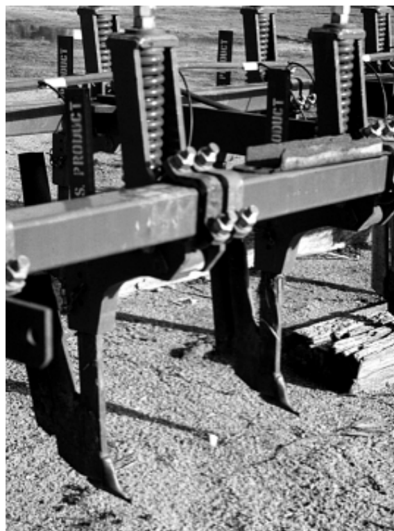
Figure 4 Check tubes & seeding boots of seeders with an undercarriage modified to handle trash.
