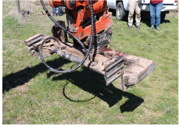
Figure 25. The Kubota head used to squeeze and lift the vine straight up out of the soil.
