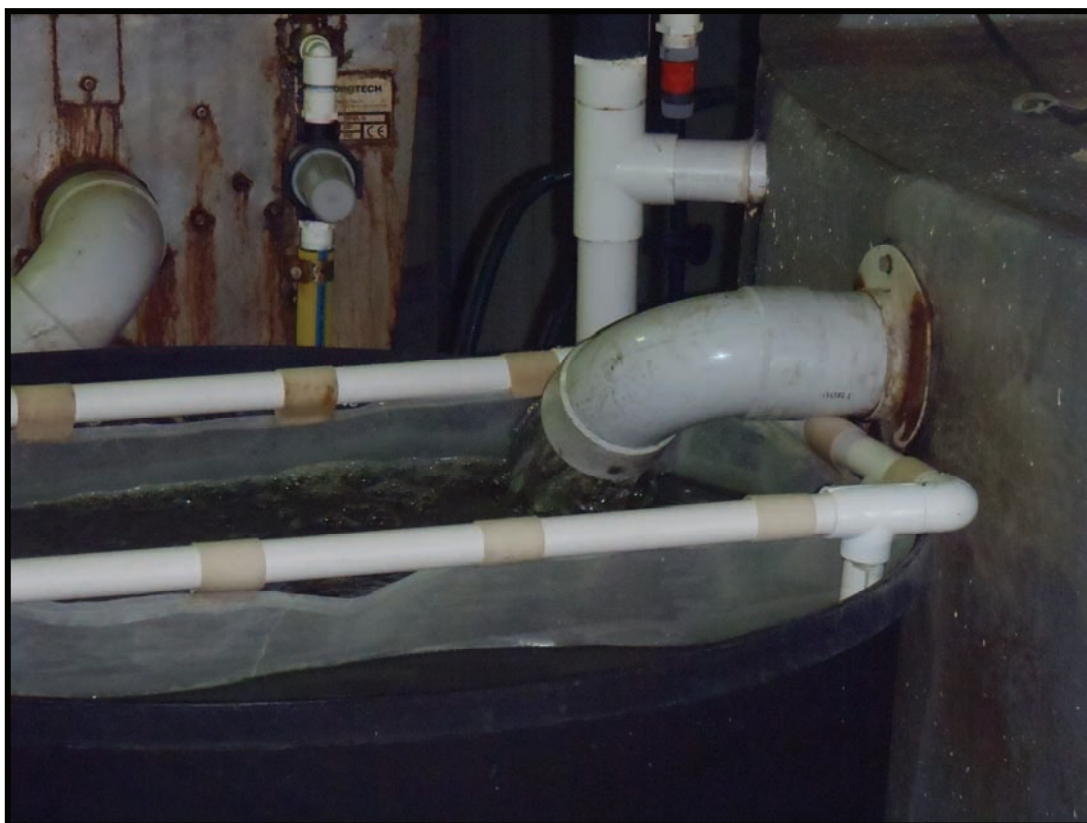
FIGURE 19: Automatic 500 µm screen egg collector mounted in a 500L sump on the outer wall of spawning tank.
