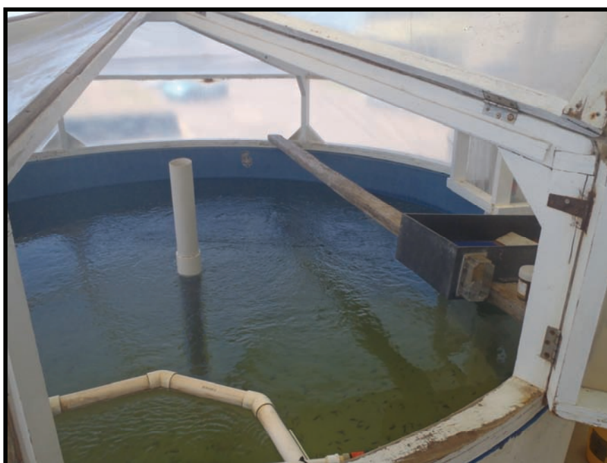
FIGURE 68: 10,000-L larval rearing tanks at PSFI. Tanks are covered with translucent, polyethylene sheeting.
