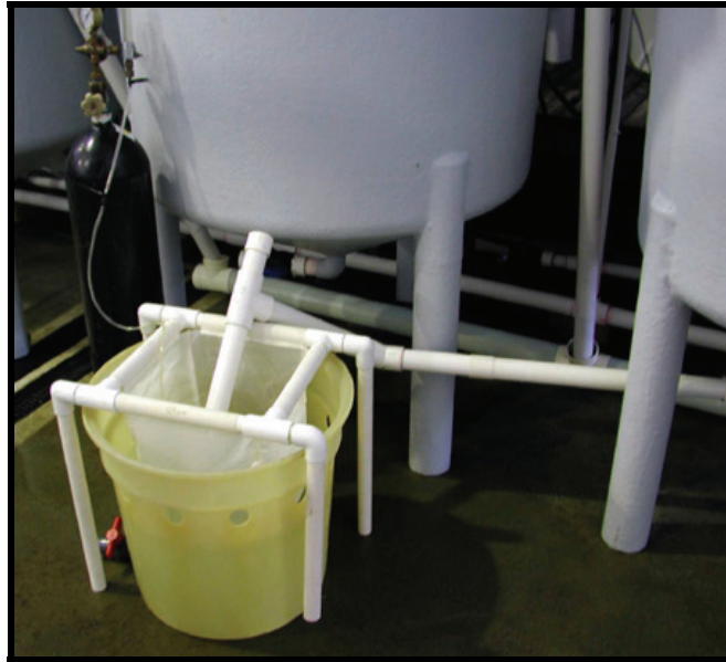
FIGURE 23: Harvester for collecting newly hatched larvae from incubation tanks. (Source Partridge et al., 2003)
