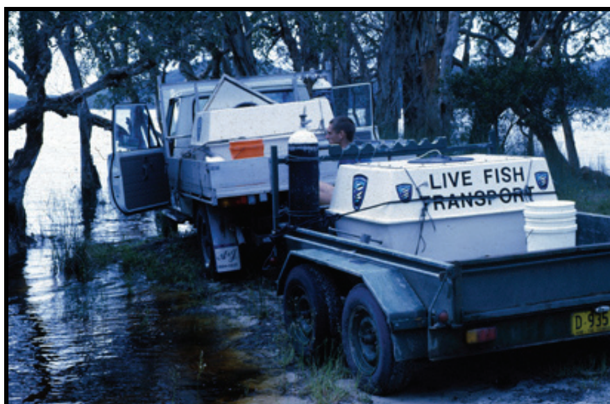
FIGURE 49: The PSFI fish transport tank with compressed oxygen bottle.
