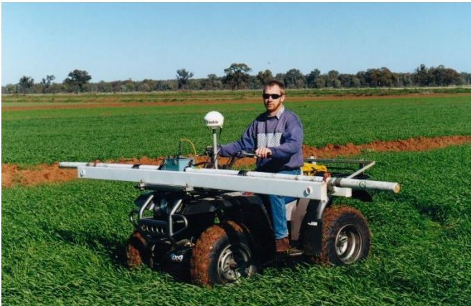
Brian Dunn using the EM31 to test for rice soil suitability
